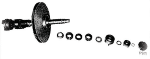
D. Outboard rotating element components removed, illustrating disassembly order.
