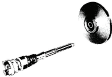
F. Impeller removed from outboard rotating element. G. Removing bearing from shaft using conventional puller.
